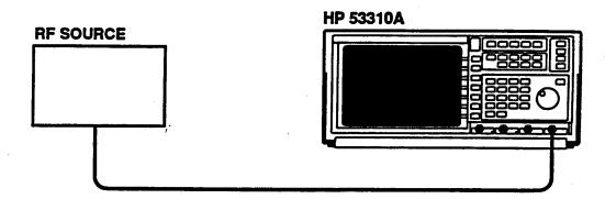
1 Set the RF source to output a power level 30 dB below the nominal power level of the transmitter (as determined in the previous section) and at the same frequency as the transmitter.
